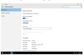
2. Set the device's date and time, time zone, and display format here.
